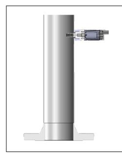
Screw the sensor with the G 1/2" thread pressuretight into the line to be measured via a connecting piece.
