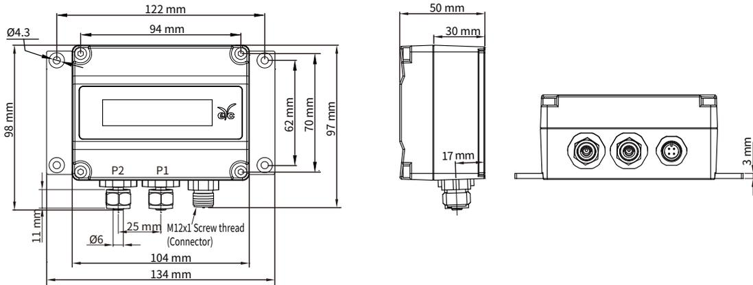
※P1 / P2 : Connected to Ø6 PVC / PTFE compressed air pipe
