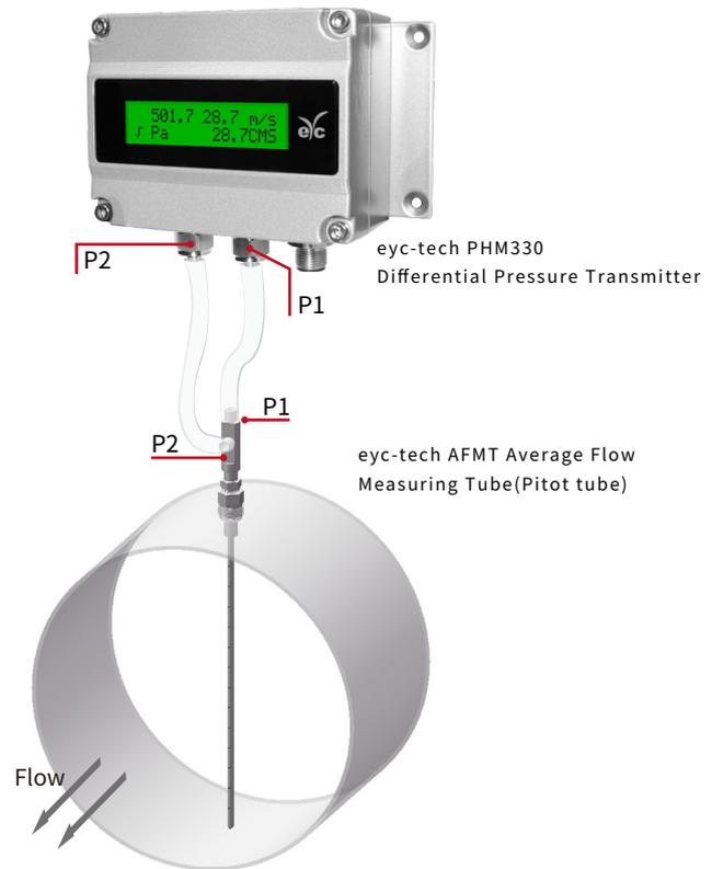
Note : The opening direction of holes on probe should be parallel to flow direction
