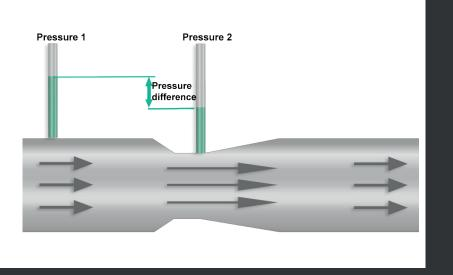
Fordifferential pressure measurement, two separate lines lead to a differential pressure measuring cell. One pressure connection (pressure 1) is located at the inlet of the Venturi tube and a second pressure connection is located at the outlet of the Venturi tube (pressure 2). Without flow, the pressure at the inlet and outlet is identical.
