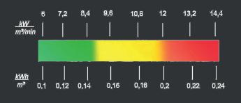
A typical specific power requirement of an oil-injected compressor can be as follows:
