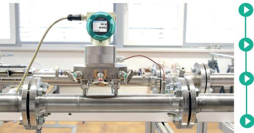
**Reference measuring device** for blower and compressor test benches (effective delivery capacity)
